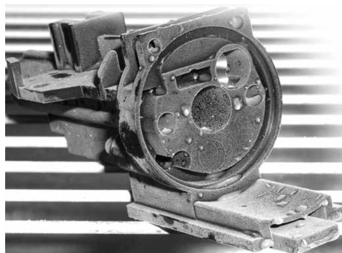
Air-storage of a component / cold test at -40 °C
