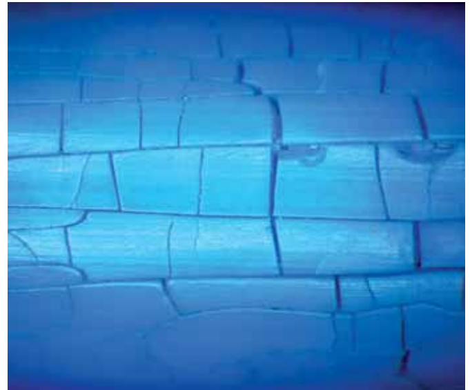
Cracking in a polyurethane tube through media exposure (Stereo microscope) (40 : 1)
