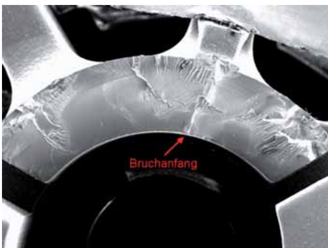
Stress cracking (brittle fracture) in an ABS plastic part (15 : 1)
