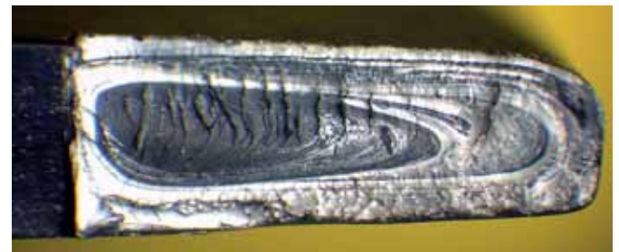
Plastic- brittle fracture and stress whitening in an ABS plastic
